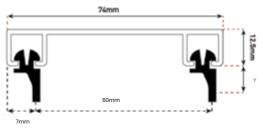
Mounted directly onto the ceiling. Pre-drilled holes every 15cm.
