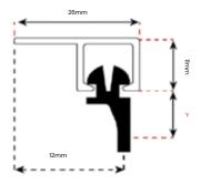
Mounted directly onto the ceiling. Pre-drilled holes every 19cm.
